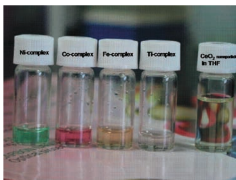
Figure 10. Perfect dispersion of nanoparticles in organic solvents.
